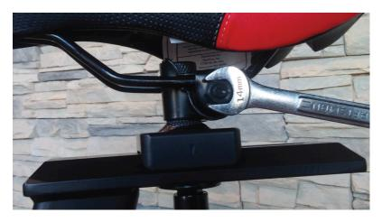
Loosen the seat clamp nut underneath the seat.
