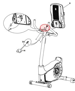
Remove the console and inspect the cable within the red circle.
