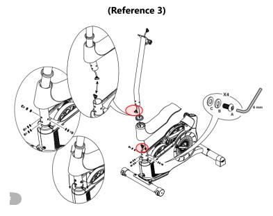
Remove the 4 bolts from the mast to remove the mast from the frame and inspect the cables.
