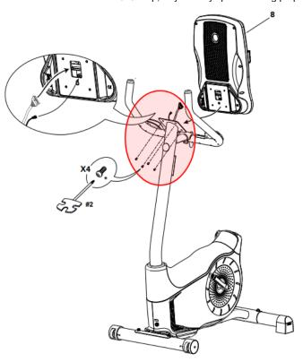
The screws attaching the console to the mast are on the back side of the console, circled in red in this image. Remove the screws to remove the console from the mast.
