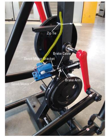
The mast to servo cable is highlighted in yellow. Inspect the entire length for damage and a secure connection.
