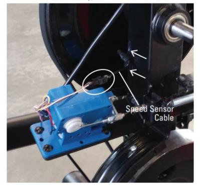
The speed sensor is located on the frame between the two white arrows. Inspect the speed sensor and the speed sensor cable for damage. Unplug the connection circled in white and securely reconnect.
