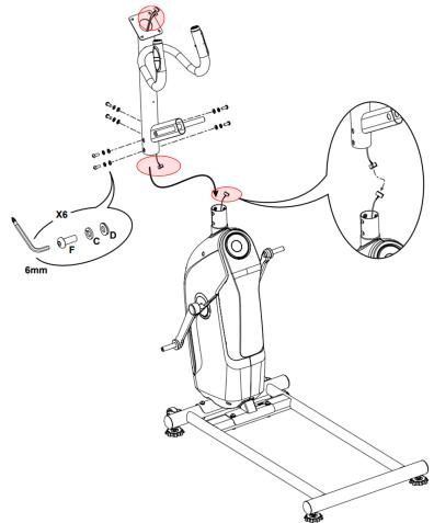
Inspect the 10-pin cables circled in red for damage.
