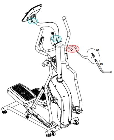
The bolts circled in red need to be removed to access the cables between the console and the console mast. Inspect the cables circled in teal for damage.
