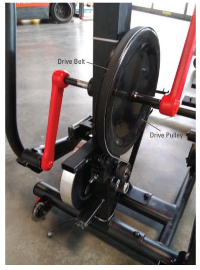
The drive pulley is the large black wheel. Rotate the drive pulley listening for noise.
