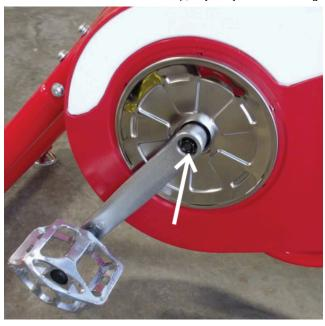
Remove the crank cap from the crank arm and tighten the lock nut shown.
