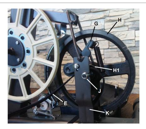
The Flywheel Pulley is labeled 'H1'.
