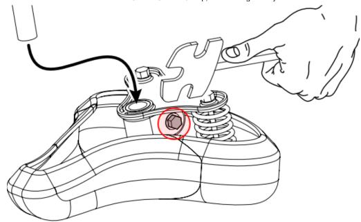
The Seat Clamp Bolts are located underneath the seat, on either side of the seat's stem. The bolt on one side is circled in red - make sure to tighten the bolts on <u>both</u> sides.
