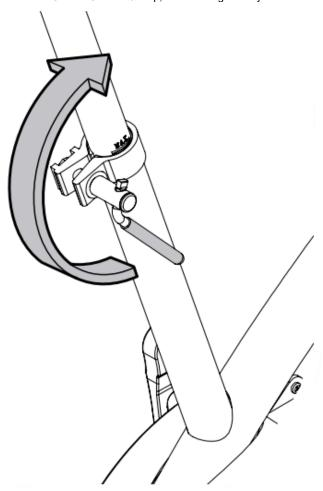
The handlebar post clamp is located on the handlebar post and should be oriented so that the inner ridge rests on top of the posts from the frame assembly.
