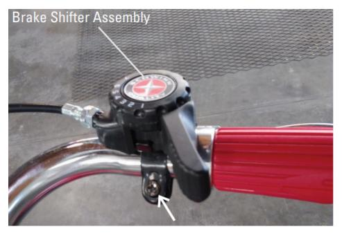
The thumb shifter (brake shifter) is located on the right handlebar and can be tightened using the screw indicated in this image.
