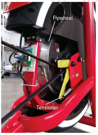
The belt tensioner (highlighted in yellow) is located next to the flywheel and maintains the tension of the drive belt.
