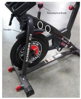
Loosen and remove the screws from the fender (circled white), taking care to hold the fender to prevent it from dropping.
