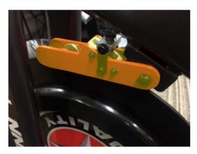
*The red magnetic brake arm (highlighted yellow) is located above the flywheel. Watch this part for movement while adjusting the Resistance Adjustment Knob.*
