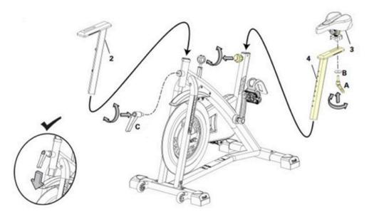
The Seat (3) should be secured onto the Seat Post (4). Tighten the Seat Adjustment Knob (A) by turning the handle clockwise until fully tightened. Tighten the Seat Clamp Bolts using the 15mm/17mm wrench included with your machine until fully tightened.
