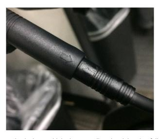
The main connection is shown with both arrows aligned and the wires fully plugged in.
