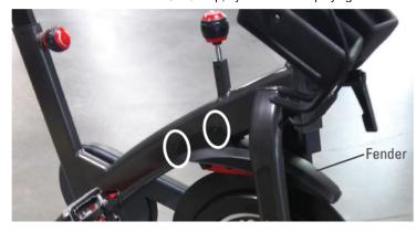
Remove the screws circled in yellow to remove the fender.
