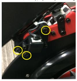
The three yellow circles indicate the location of the screws to remove in order to access the Resistance Sensor Magnet.
