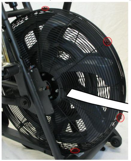
Remove the screws located along the seam of the fan cover. The screws are spaced evenly around the entire seam; the screws visible in this image are circled in red.
