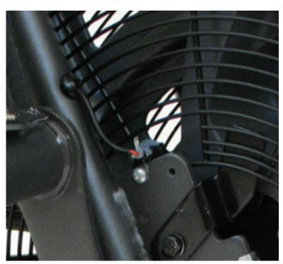
A properly positioned speed sensor should look just like this image.
