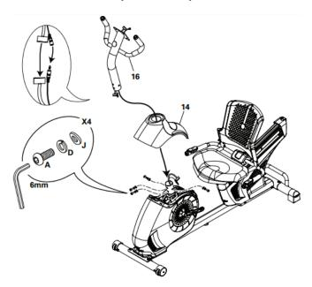
The console is attached to the mast by 4 bolts. Remove the 4 bolts with a 6mm Allen wrench and carefully lift the console up to expose the cable connections.
