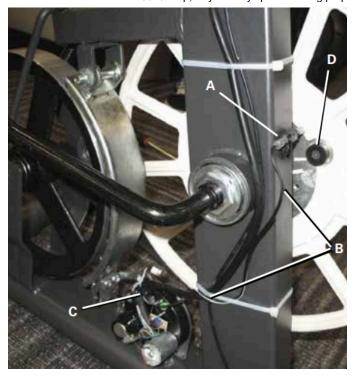
Inspect the RPM sensor magnet (D) and ensure it is securely in place and undamaged.
