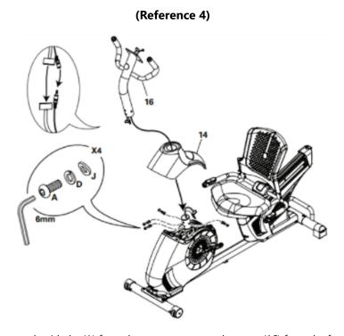
Remove the 4 bolts (A) from the mast to remove the mast (16) from the frame.
