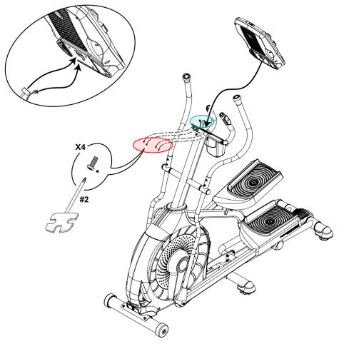
The screws circled in red need to be removed to access the cables between the console and the console mast. Inspect the cables circled in teal for damage.
