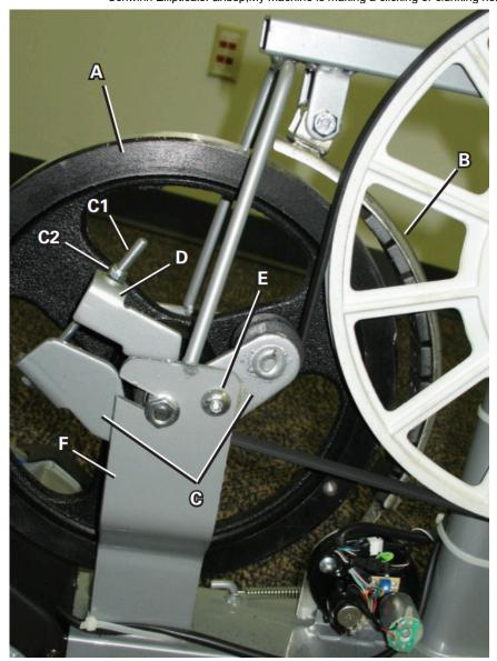
The drive pulley is pictured on the left side (white wheel with spokes). Rotate the drive pulley and listen to the flywheel (black wheel labeled 'A').
