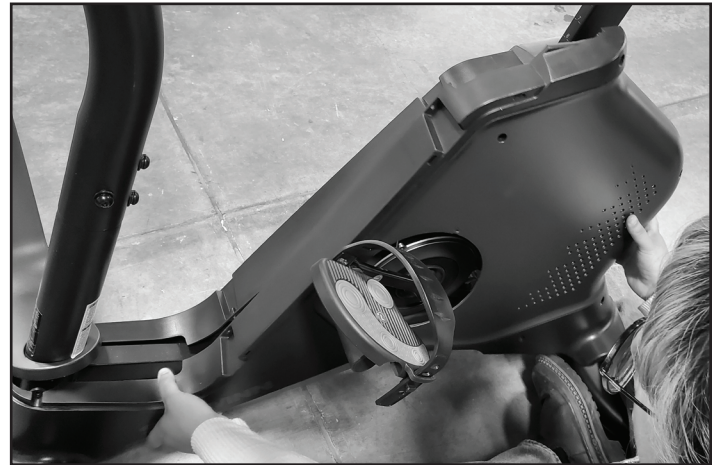
Left shroud removed (Crank disc not shown for clarity)
