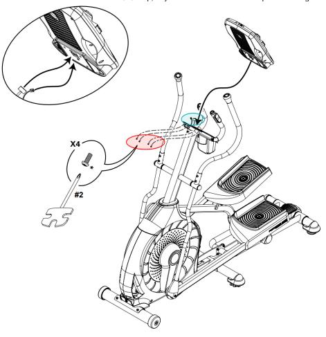
The screws circled in red need to be removed to access the cables between the console and the console mast.
