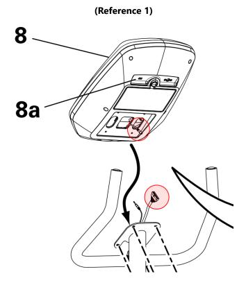
Inspect the circled cable connections, reseating if undamaged.
