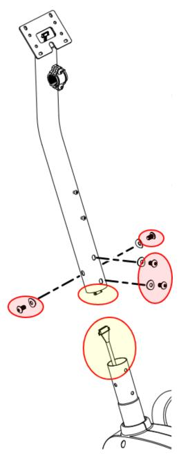
Remove the screws circled in red and inspect the newly exposed cable connections.
