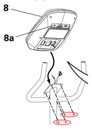
Remove the 4 screws indicated from the back of the console, then remove the console from the mast.
