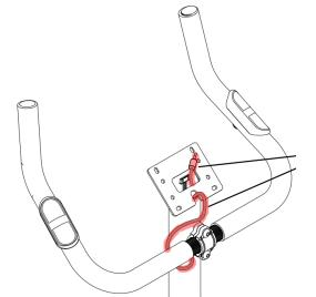
Remove the handlebars and inspect the cable within (highlighted red).
