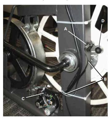
The RPM Sensor (A) is located on the frame of the bike. Inspect both the sensor (A) and cable (B).
