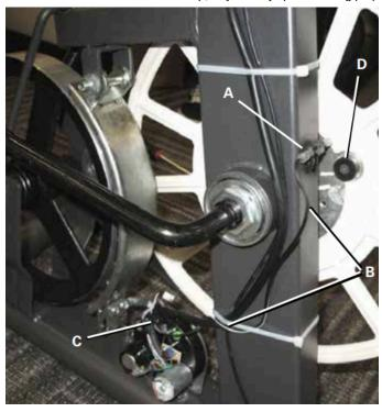
Inspect the RPM sensor magnet (D) and ensure it is securely in place and undamaged.
