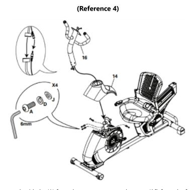
Remove the 4 bolts (A) from the mast to remove the mast (16) from the frame.
