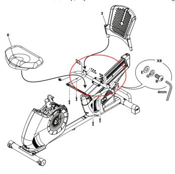
There are 8 bolts connecting the seatback to the static handlebars, circled in red. Remove the bolts using a 4mm Allen wrench and then slid the seat back out of the bracket. The heart rate wire is located in the handlebar.
