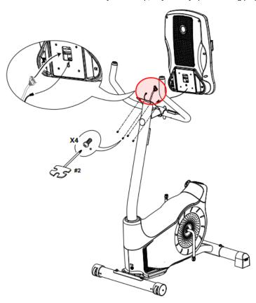
The screws attaching the console to the mast are on the back side of the console. Remove the screws to remove the console from the mast and inspect the cable.
