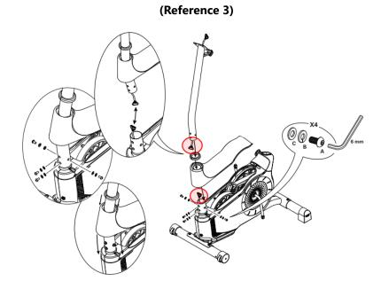
Remove the 4 bolts from the mast to remove the mast from the frame. Inspect both sides of the cable connection, circled in red.
