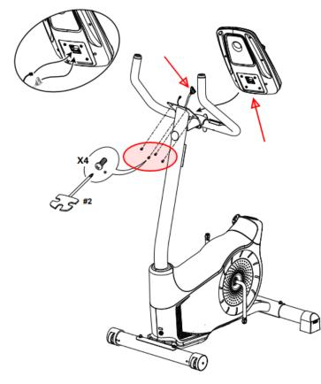
The red circle indicates the screws to remove. Remove the console and inspect the cables indicated by red arrows.
