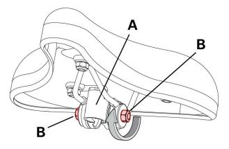
Tighten both seat clamp nuts (B, highlighted red) to secure the seat to the seat post. Image may not match your bike exactly - the BowFlex C6 is shown in this image.
