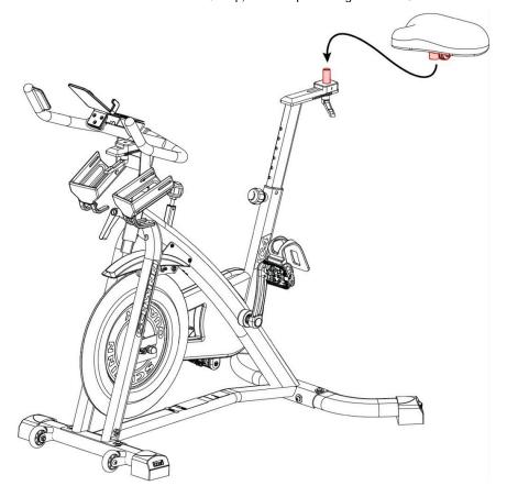
Attach the seat to the seat post by sliding the seat bracket over the post (both highlighted red).
