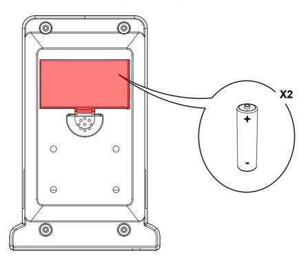
The battery compartment cover is highlighted in red. Replace the existing batteries with two new AA-sized batteries.
