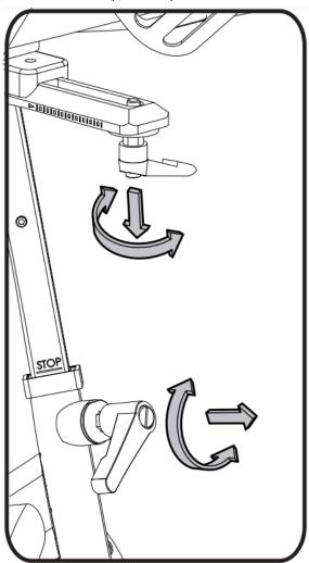
The Seat Adjustment Knob is located underneath the Seat. Turn the handle clockwise to tighten the Seat.
