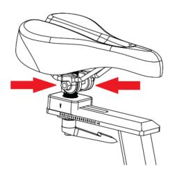
The Seat Clamp Bolts are located underneath the seat, on either side of the seat's stem.
