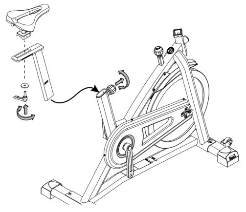
The Seat (3) should be secured onto the Seat Post (4). Tighten the Seat Adjustment Knob (A) by turning the handle clockwise until fully tightened. Tighten the Seat Clamp Bolts using the 15mm/17mm wrench included with your machine until fully tightened.
