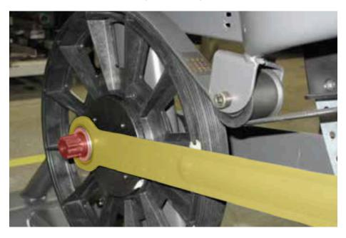
The crank to pulley junction (crank link) is highlighted red and the crank linkage arm is highlighted yellow.
