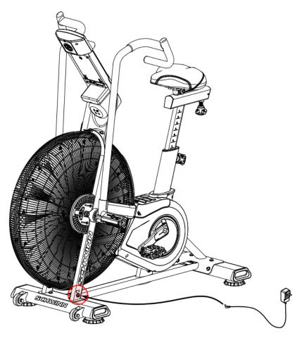
The power inlet plug is located on the lower left side at the front of your bike, near the base of the frame.
