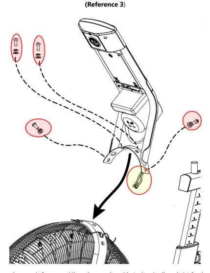
Remove the console from your bike to inspect the cable (red and yellow circle) for damage.
