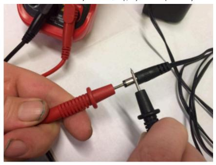
The voltmeter should be set up as shown to read the voltage of the power adapter.
