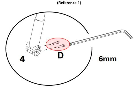
Remove the 2 screws at the bottom of the handlebar as shown.
