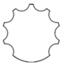
The opening of the handlebar and the axle of the pivot shaft is shaped so installation can only be performed one way. The opening/axle has 7 points at the top and a smooth, curved bottom.
