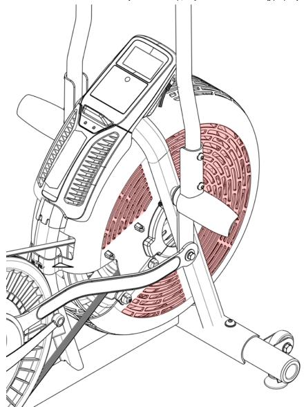
Inspect the belt through the holes in the fan cover
