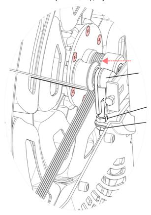
Loosen the hardware shown (6 screws), adjust the fan position, then re-tighten the hardware.
